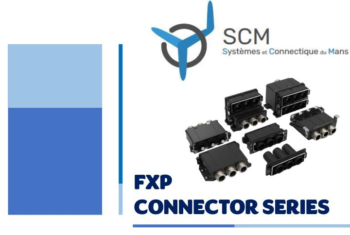
Rugged power connectors for all mission critical power applications on rolling stock, meeting EN 50467 including requirements for fire and smoke compliance per EN 45545-2. Allowing multiple combinations with just ten variants this connector series saves weight, space and contains more electrical capacity up to 650 amps, 4000 volt.
